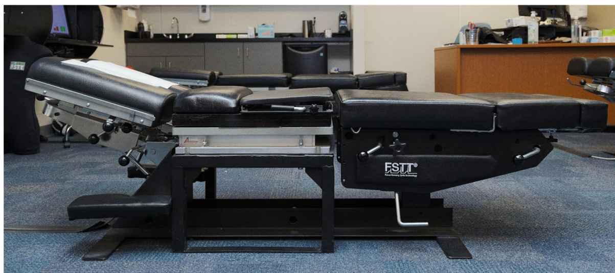
Figure 2. The FSTT® system, equipped with a modified Elite Stationary treatment table with drop-pieces and an embedded AMTI force plate.
